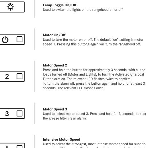
Used to select the strongest, most intense motor speed for superior extraction. This speed will only run for 6 minutes, and after 6 minutes it will return to the last set motor speed. If it is activated with the motor turned off, the hood will switch to OFF at the end of the time.
