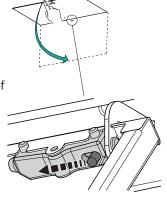
6. Remove the frame by unfastening the 4 screws (2 on the right and 2 on the left).
