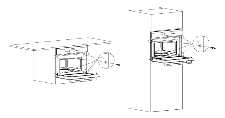
Note: Do not take the door handle as force bearing point during the installation and removal.
