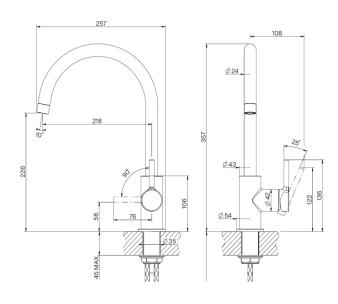
**PLEASE NOTE:** Large and heavy taps should ideally be mounted directly through the solid benchtop or fully supported from underneath. For all other swivel taps, we recommend the use of the Franke Tap Support Arm to provide additional support. Please ensure all Franke tapware is installed at a pressure of no greater than 500 kPa in accordance with AS/NZS3500 and insist that your plumber flushes all of the water supply lines before installing tapware. Failure to do so may void warranty.
