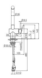
**PLEASE NOTE:** Large and heavy taps should ideally be mounted directly through the solid benchtop or fully supported from underneath. For all other swivel taps, we recommend the use of the Franke Tap Support Arm to provide additional support. Please ensure all Franke tapware is installed at a pressure of no greater than 500 kPa in accordance with AS/NZS3500 and insist that your plumber flushes all of the water supply lines before installing tapware. Failure to do so may void warranty.
