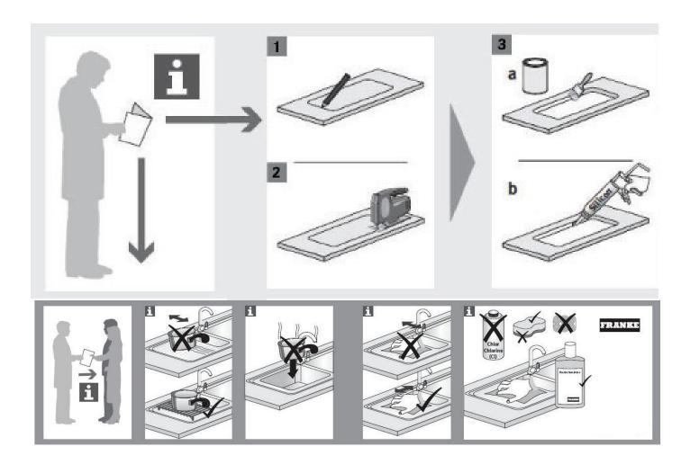
Please note: Top mount only. No install clips required. Please do a bead of silicone and push down firmly.
