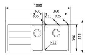
NOTE: Tap and pop-up waste control holes are part pre-drilled on the underside of the Fragranite Sinks, for knocking out as required
