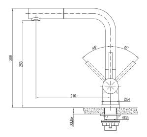
\*56mm is the **minimum distance** required between the tap base and a splashback/ wall directly behind the tap in order for the tap to operate correctly.
