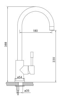
**PLEASE NOTE:** Large and heavy taps should ideally be mounted directly through the solid benchtop or fully supported from underneath. For all other swivel taps, we recommend the use of the Franke Tap Support Arm to provide additional support. Please ensure all Franke tapware is installed at a pressure of no greater than 500 kPa in accordance with AS/NZS3500 and insist that your plumber flushes all of the water supply lines before installing tapware. Failure to do so may void warranty.
