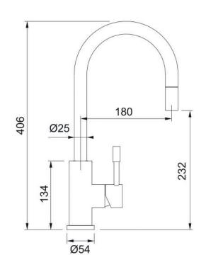
\*56mm is the **minimum distance** required between the tap base and a splashback/ wall directly behind the tap in order for the tap to operate correctly.
