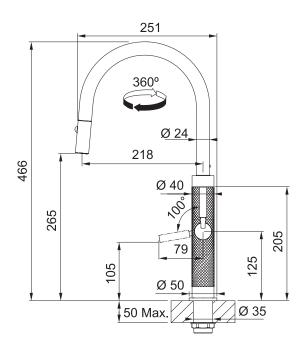
**PLEASE NOTE:** Large and heavy taps should ideally be mounted directly through the solid benchtop or fully supported from underneath. For all other swivel taps, we recommend the use of the Franke Tap Support Arm to provide additional support. Please ensure all Franke tapware is installed at a pressure of no greater than 500 kPa in accordance with AS/NZS3500 and insist that your plumber flushes all of the water supply lines before installing tapware. Failure to do so may void warranty.
