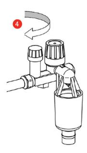
4 Connect the Waste T-piece (6) to the Inlet Pressure Relief Valve and Tundish (4) using the Flexible Plastic Hose (7). The Tundish has a water trap in order to prevent odours from escaping from the waste pipe.
